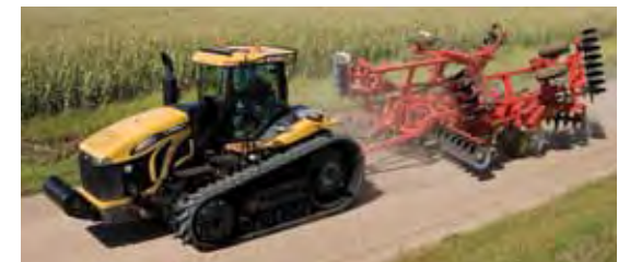
Featuring the highest transport speed of any track tractor, the Challenger MT800C Series travels up to 24.6 mph (39.6 kph) for quicker moves between fields and more productivity per day.
