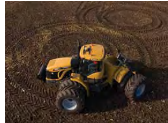
A 42-degree turn angle provides the shortest articulated turning radius in the industry, allowing for tight maneuvers on headlands and corners.
