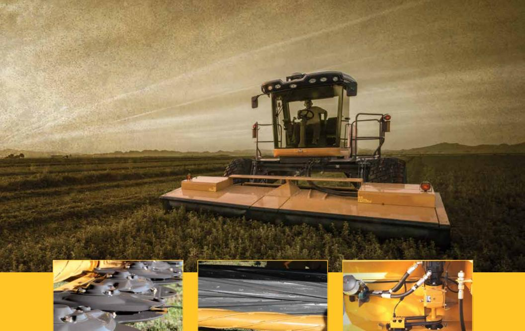
Our RazorBar™ cutter bars feature a low-profile, spur gear cutterbed that's thinner in design for closer cutting – so you can slice through lush alfalfa, tangled grass and tall Sudan with ease.
